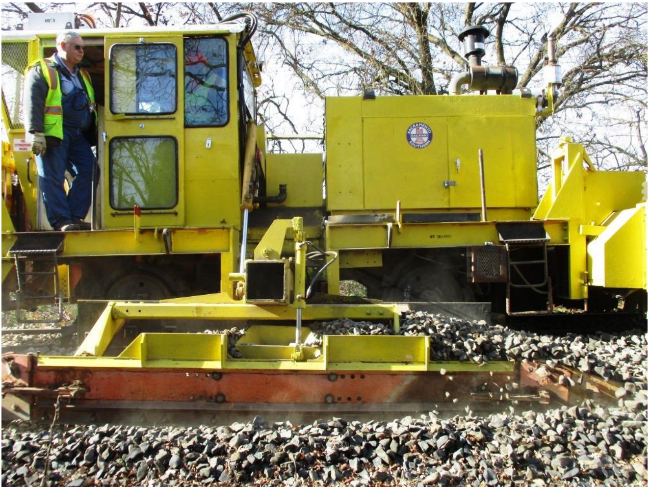
Chris keeps an eye on the redistribution of rock as Ed pilots the regulator up the hill
